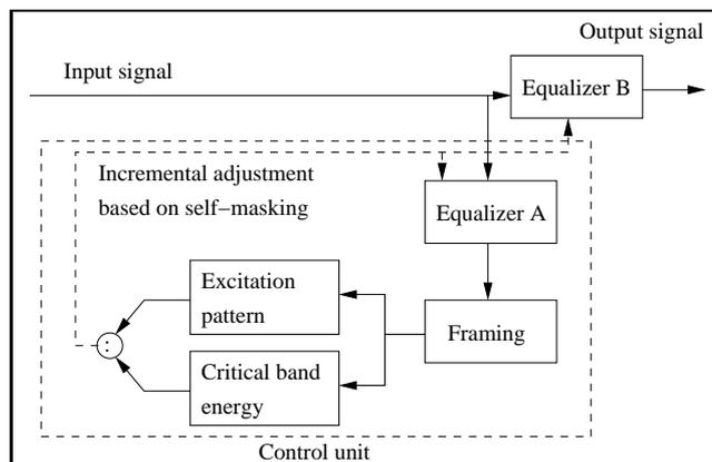
**Figure 1.** Outline of the automatic equalizing method. A control unit adapts the equalizer settings in order to reduce the self-masking that is determined by the ratio between the excitation pattern and the signal energy within each critical band.
